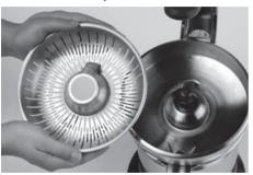
Place the juicing cone onto the drive shaft and press down lightly to lock the cone into position.
